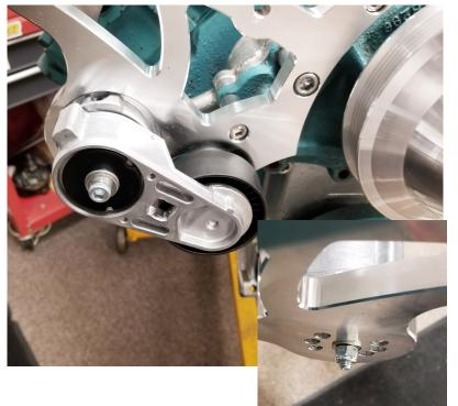
Install (P758A-04) tensioner to a/c bracket with a (S162) 5/16-18 x 3" shcs and two (S660) 5/16 washers and secure with a (S616) 5/16-18 lock nut. There are three positions the tensioner can be installed in. We recommend installing with the tensioner in the middle position.
