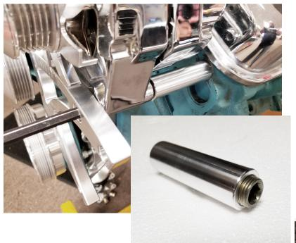
First thread (S453) 5/8-18 x .850" set screw in to alternator support spacer (30142-A). Now install alternator to main bracket with alternator spacer in between alternator and cylinder head. Adjust (S453) set screw to take up any gap. Secure with a (S282) 3/8-16 x 6" shcs
