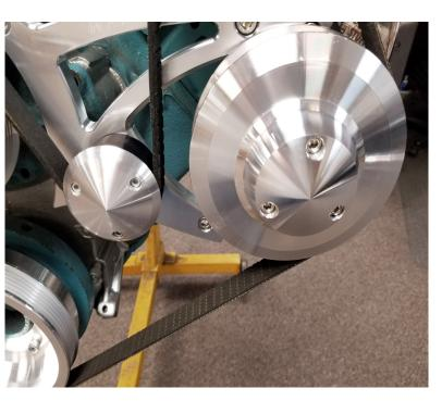
**Step 19** Install (302-A) idler pulley nose cover to (740-A) idler with three (S022) 8-32 x .375" shcs.
