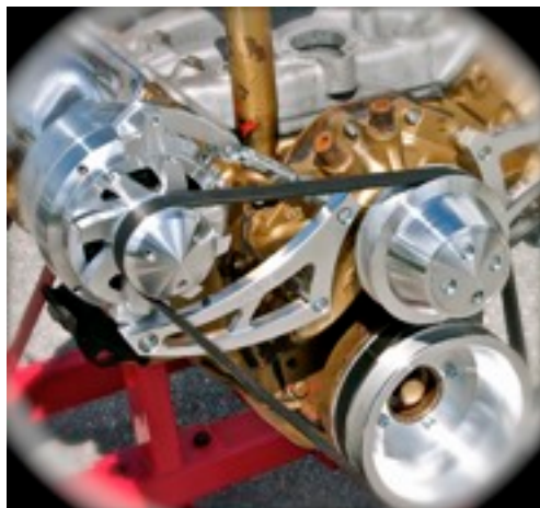
Installed Alternator Bracket
