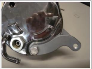
Now mount the pump to the lower bracket as shown, use a (TP3-.750) spacer between the front support and the lower support and a (TP3-.800) spacer between the rear support and the lower support. Securing with a (S266) 3/8" x 3" SHCS as shown.
