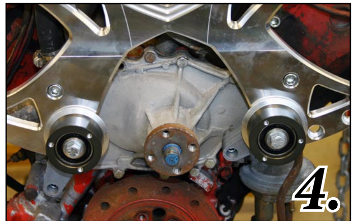
Photo 3 Install the Front Main Plate (17001-A) to the rear supports using (4) \frac{3}{8} x 1" SHCS (S248) through the main plate and into the left and right spacer brackets.
