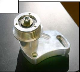
**PHOTO-9.** Installing the Idler and Bracket assembly to the water pump. Use (3) AC3-.500 Alum. Spacers between the water pump and the bracket, use the (3) ? 8 x 120mm SHCS (S557) to mount the bracket As shown. Install the Idler cover (302-A) With the (3)  $\frac{8}{32}$  x  $\frac{3}{8}$  SHCS (S022).
