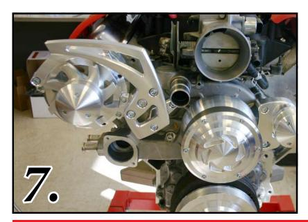
**PHOTO-7** Install the Alternator using (1) <sup>3</sup>/<sub>8</sub> x 3" SHCS (S266) in the lower Hole and (1) <sup>5</sup>/<sub>16</sub> x <sup>7</sup>/<sub>8</sub>" SHCS in the upper hole (S144) **NOTE: if using a Chrome Alternator the top bolt will be a ? 8 x 20 MM SHCS (S540)** Replacing the <sup>5</sup>/<sub>16</sub> x <sup>7</sup>/<sub>8</sub>" SHCS. Tighten all bolts at this time.
