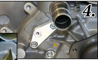
**PHOTO-5.** Install the Rear Alternator Support Bracket (20051-B) to the tapped outer hole of the water pump using (1) ? 10 x 30mm SHCS (S561). *Leaving loose at this time.*
