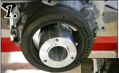
**PHOTO-1**. Remove 16mm O.E.M. bolt from the crank. Install the appropriate March Crank Adapter Hub for your LS-1 motor. Apply Loc - Tite to the threads of provided ? 16 x 130mm Hex Bolt (S569) and using a "/16" i.d. washer (S686) secure Adapter Hub and crank pulley, torque to 90 ft lbs.
