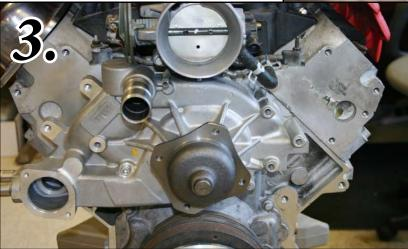
**PHOTO-3.** Apply silicone sealer to both sides of the water pump gaskets and install the provided Water Pump (P116).
