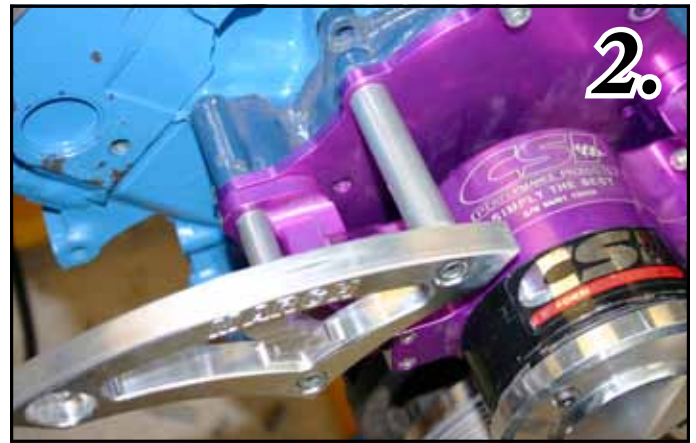
Photo-3 Installing the Ford Alternator. Use a TP7-2.560 Spacer Between the Alternator unit and the head. and a \frac{7}{16} x 6\frac{1}{2} " SHCS (S378).
