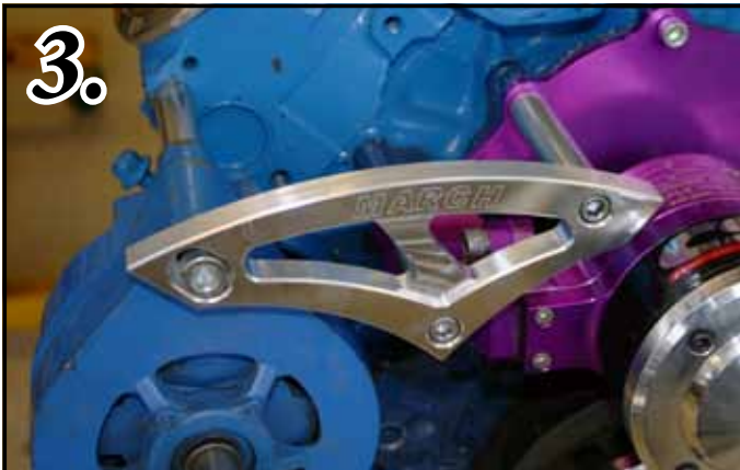
Photo-4 Installing the Alternator. Adjustment rod (RA-1.625), Thru the lower timing cover hole in the motor use a \frac{5}{16} x 4" SHCS (S170) and space with a AC3-1.250 Spacer. Now attach the 2\frac{1}{2} " Rod to the Alternator with a \frac{3}{8} x 2\frac{1}{2} " SHCS (S262) and use a AC3-1.250 Spacer Between the Alternator and the Rod.
