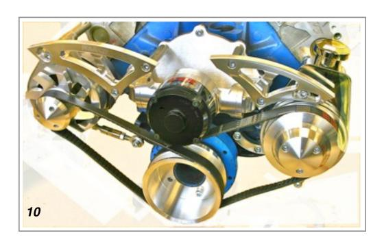
Make Sure All Bolts Are Tight Run motor at Idle for five Minutes and Re-Check (Note) this is a single wire Alt Set UP and requires a ground strap for proper operation
