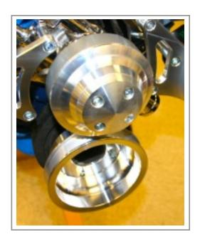
**Photo-11**Mount the (395-A) A/C Clutch Cover with three 1/4" Button Head Bolts (S124).
