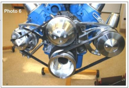
Note: 36" P/S Belt is a tight fit and will require the bolt to be removed from slot to install belt.
