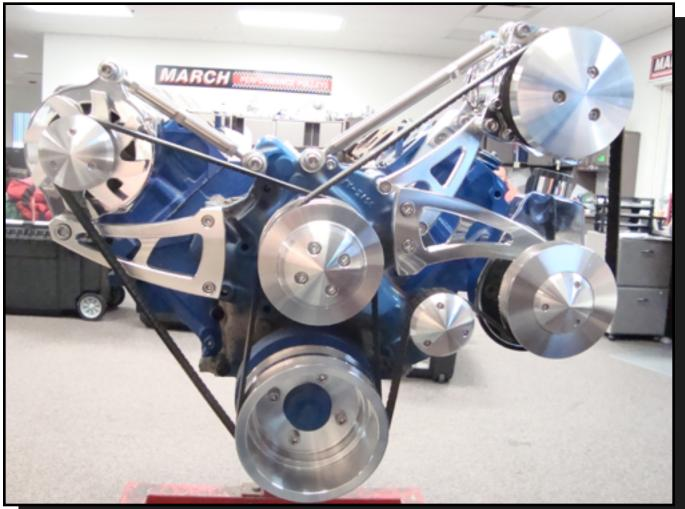
Ford 460 Alternator, Air Conditioning & Power Steering
