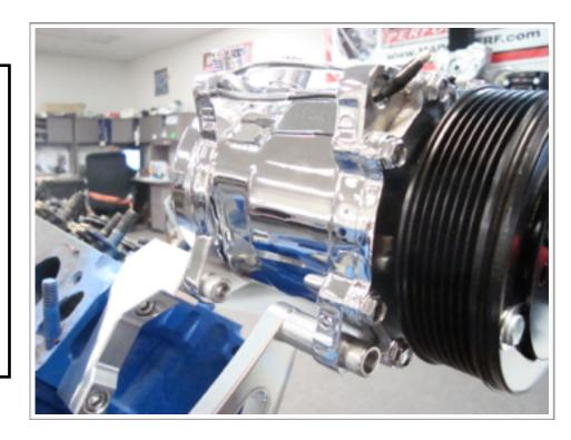
Mount the (RA-8.000) adjust rod to the water pump with one 3/8" x 1" SHCS (S248). Tie the other end to the top left ear using one 3/8" x 2" SHCS (S256) and place a (TP3-.400) spacer between the back of the ear and the adjustment rod. Tighten with a 3/8" lock nut (S622).
