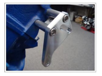
Install the power steering rear support bracket (30211-B) to the two outer head holes with two (TP7-1.625) spacer tubes between head and bracket and tighten with two 7/16" x 2-1/4" SHCS (S356).
