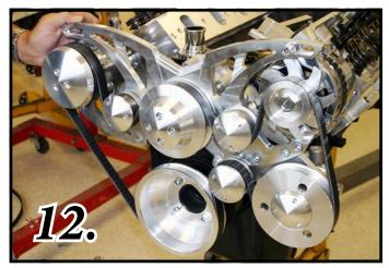
Fig 13: Slip the supplied (30436) March Adjustment Tool over the two (MM100) bushings at the Alternator an A/C sides. Use a wrench to turn the adjustment tool outward to tighten the serpentine belt to 100 ft. lbs. Use the holes in the adjustment tool to tighten both M8 socket head cap screws when correct belt tension has been achieved. Remove the adjustment tool and keep for future use.
