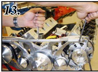
TIP: Fig-13a: Your Serpentine belt is tight when it can't be moved by more then 1/2 inch at it's longest span between pulleys. The belt should not be able to be twisted by more then half a turn.
