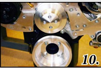
*Fig 11:* Install Alternator Fan (221-A) and Alt Pulley (206-A). Slide the fan over the shaft followed by Alt Pulley and Lock Washer (S685). Use an impact gun to torque the alternator lock nut. Now install the Alt cover (306-A) with (3)  $\frac{8}{32}$  x 1" SHCS (S028).
