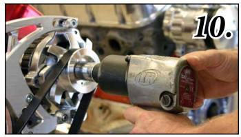
**Fig-11** Install the Power Steering Pulley (629-A) with the lock nut and then install the cover (360-A) with (3)  $\frac{1}{4} \times 1\frac{1}{4}$ " SHCS (S106).
