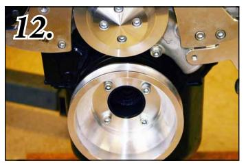
Fig 13: Install Dayco Belt (5060675) 67.5" wrapping as shown.
