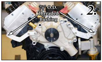
**FIG-3** Install the Main Face Plate (30451-A) See Diagram and install the main face plate using the following bolt Sizes and spacers.
