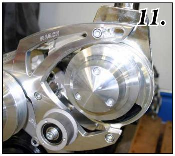
*Fig 12:* Install Crank Pulley (2236-A) with (4) 3/8 x 1" SHCS (S248).
