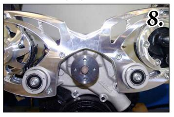
**Fig-9** Use the Adapter ring  $^{3}$ /4" O.D. x  $^{5}$ /8" I.D. (S716) over the water pump shaft and install the water pump pulley (2232-A) and the water pump nose cover (312-A) with four  $^{5}$ /16 x  $^{7}$ /8" SHCS (S186).
