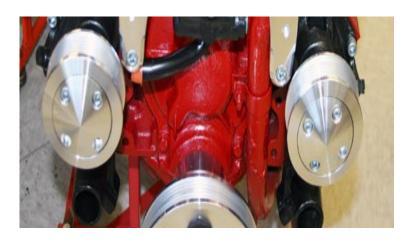
**Step-13** Install the two (2072-A) water pump pulleys and the two (329-A) water pump pulley caps using the eight provided 5/16- 24 x 1 1/4" SHCS (S189).
