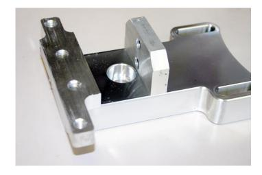
**Step-4** Mount the rear alternator & a/c support bracket (30602-B) using two 3/8 x 11/4" (S250) shcs as shown but leave loose for adjustment later.
