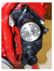
**Step-2** Make sure the sealing face of the coolant outlets are clean, flat and free of old gasket material. Install the two water pumps (P138) & (P139) (45 Deg) or (P136) & (P137) (90 Deg.) Using (2)  $3/8 \times 1 \ 3/4$ " shcs (S254) for the center bolts and two  $3/8 \times 1$ " shcs (S248) for the outer bolts. The inner bolts holes will use the two  $3/8 \times 11/2$ " Studs (S337) and the two 3.100 long stainless tapped spacers (S787) as shown.
