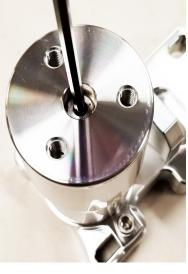
**Step-6** Install (S310) 5/16 shoulder bolt into center of idler assembly.
