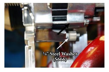
**Step-11** In the lower alternator mounting hole use a (S266) 3/8-16 x 3" shcs through the main front bracket and the lower alternator mounting ear and into the rear support bracket installing a (S666) 3/8" washer between the rear support bracket and the rear of the alternator mounting ear.
