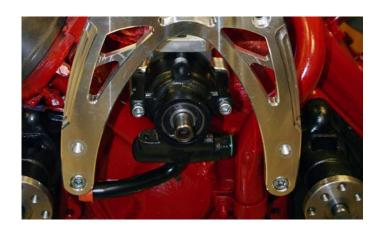
**Step-9** Install the main front bracket (30601-A) using two (S248) 3/8 x 1" shcs in the lower mounting holes to the two stainless threaded spacers on the water pumps.
