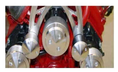
**Step-15** Install the idler pulley (655-A) using three (S144) 5/16 x 7/8" shcs.
