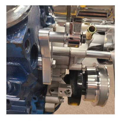
Install (P555) alternator to main bracket in upper slot using a (MM100) bolt bushing and a (S148) 5/16-18 x 1.25" shcs. In lower hole secure with a (S284) 3/8-16 x 6.5" shcs and a (TP7-3.700) spacer between alternator and rear support bracket. **Note: Before installing spacers you can use S284** 3/8 bolt to align rear support bracket to main bracket.
