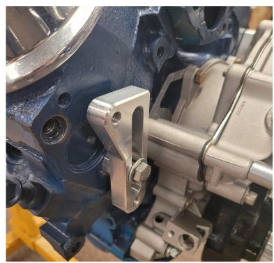
**Step 7** Install (30421-A) tensioner bracket to main bracket using two (S244) 3/8-16 x .75" shcs.
