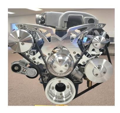
**Step 16** Once belt is on then install (759-A) tensioner cover with two (S022) 8-32 x .375" shcs
