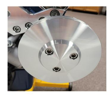
Install belt as shown in photo. use a 1/2" drive ratchet on tensioner and rotate clockwise to install belt. Kit (30805) without power steering will use a 64" 6 rib belt we recommend Dayco # 5060640. Kit (30810) with power steering will use a 67.5" 6 rib belt or Dayco # 5060675
