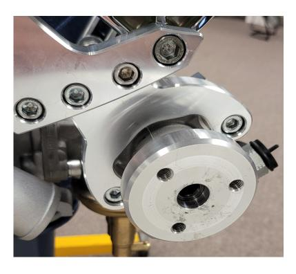
**Step 14** Install (650-A) power steering pulley to power steering pump with three (S144) 5/16-18 x .875" shcs.
