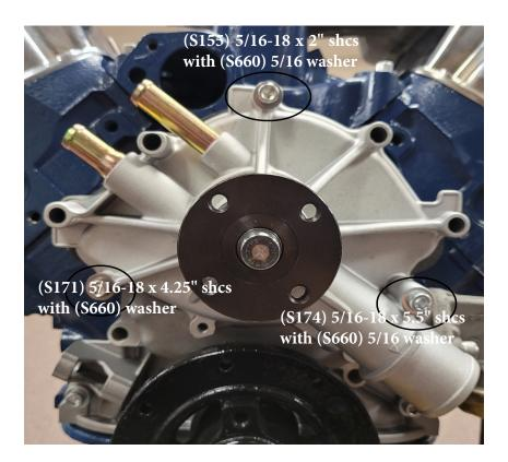
Install new (P173) water pump and gasket. At the top mount use a (S155) 5/16-18 x 2" shcs and (S660) 5/16 washer. On lower passenger side of pump use a (S171) 5/16-18 x 4.25" shcs and (S660) 5/16 washer. On lower driver side use a (S174) 5/16-18 x 5.5" shcs with (S660) 5/16 washer.
