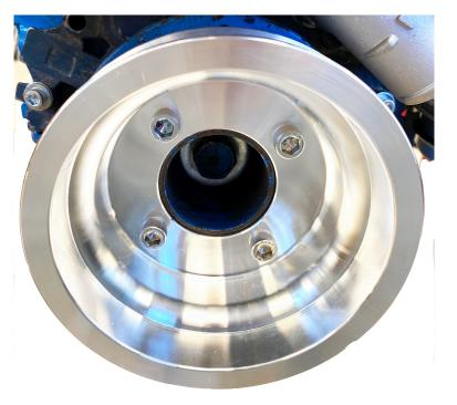
Install crank pulley (2008-A) with four (S248) 3/8-16 x 1" shcs. Note: A lot of aftermarket balancers/dampners will require crank pulley spacers to bring the crank pulley to correct alignment. March Performance carries spacers to correct. Please contact us for help.
