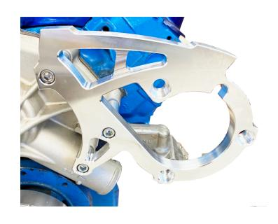
**Step-6**Mount the Ford power steering pump to bracket using three (S560) m10-1.25 x 20mm shcs.
