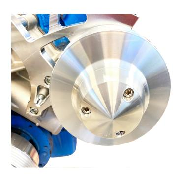
This kit requires the use of a 68" 6 rib belt. We recommend a **Dayco brand belt part# 5060680.** Recommended routing is shown in picture below. After belt has been installed and tension is applied, now install (759-A) tensioner cover using two (S022) 8-32 x .375" shcs
