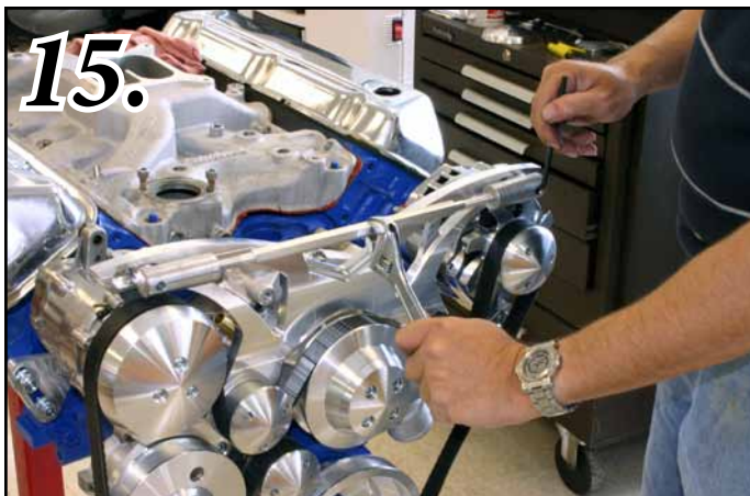
Photo 15 Slip the supplied March Adjustment Tool (BLT-12) over the two (MM100) bushings at the Alternator an A/C sides. Use a wrench to turn the adjustment tool outward to tighten the serpentine belt to 100 ft. lbs.
