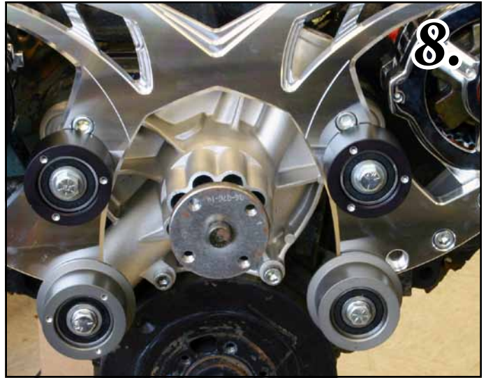
Photo-9 Install the Idler Covers (302-A) with (3) \frac{8}{32} x \frac{3}{8} " SHCS (S022)
