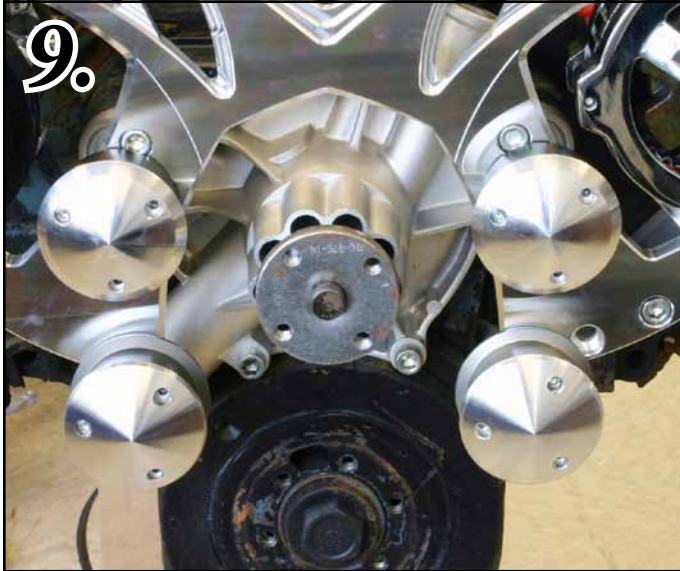
Photo-9 Install the Idler Covers (302-A) with (3) \frac{8}{32} x \frac{3}{8} " SHCS (S022)
