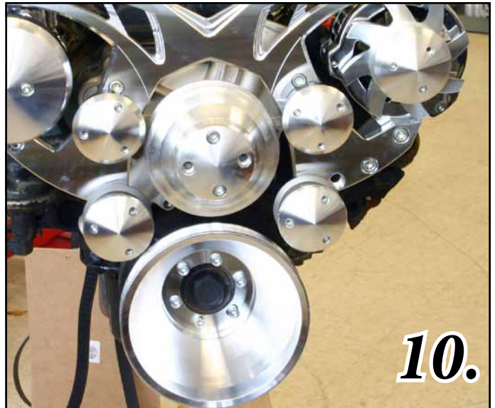
Photo-9 Install the Idler Covers (302-A) with (3) \frac{8}{32} x \frac{3}{8} " SHCS (S022)
