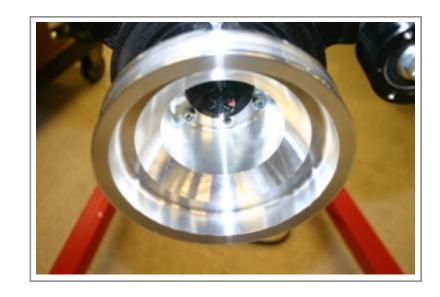
On the Alternator install the Alt. fan (221-A) the (206-A) Pulley securing with the (S685)
