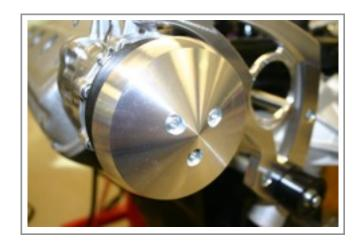
**Photo-16**Install your power steering pulley (650-A) with three 5/16 x 7/8 SHCS (144)
