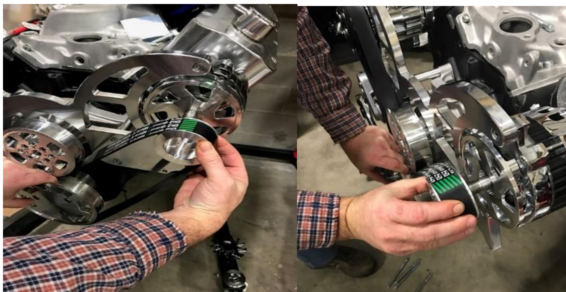
Belt Install with alternator pulley
